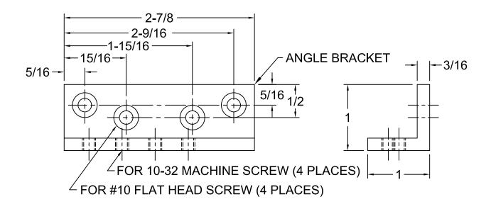
THE ANGLE BRACKET IS SECURED TO THE HEADER WITH WOOD OR MACHINE SCREWS. THE JAMB BRACKET FASTENS TO THE ANGLE BRACKET WITH MACHINE SCREWS. THE CHANNEL MOUNTS ON THE DOOR WITH SEX BOLTS. REVERSE INSTALLATION METHOD IS NOT RECOMMENDED FOR EXTERIOR DOORS OPENING OUT.
